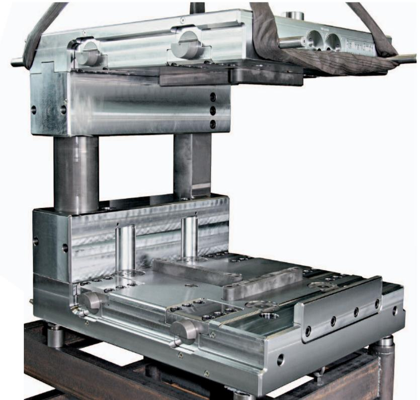
Base holder with flat/round pillar guide, fixed centring strips in the base holder lower section and adjustable centring strips in the base holder upper section, double-hydraulic cassette lifting cylinders in the base holder lower section and hydromechanical cassette wedge-type clamping elements in the base holder lower and upper sections (view from front left)
