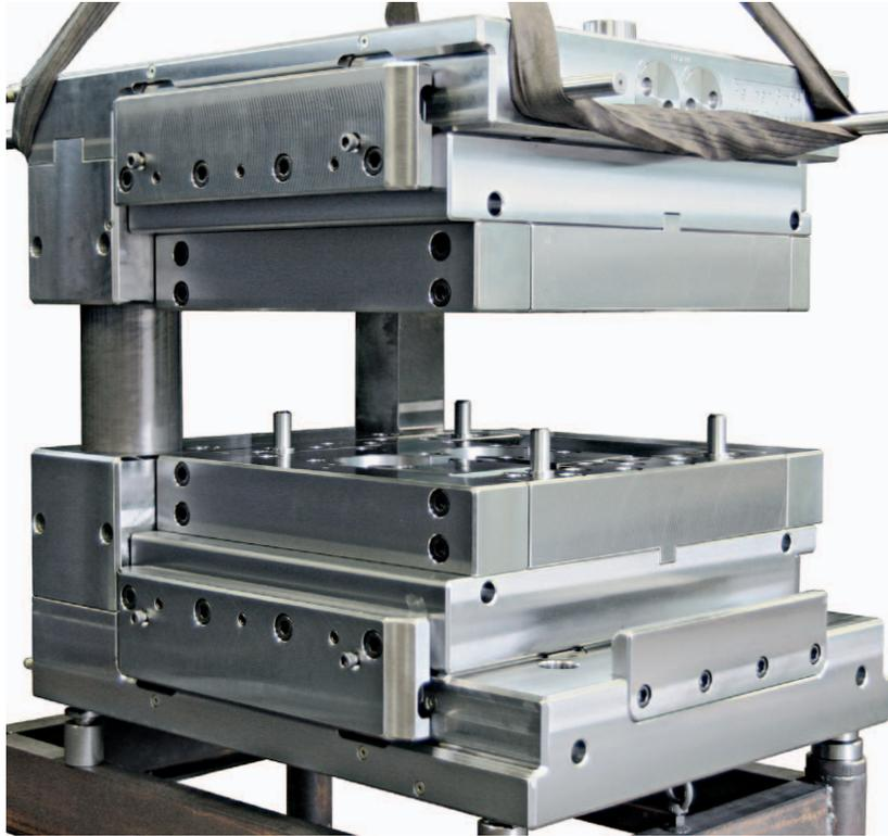
Base holder with installed, clamped rectangular / round forging die cassette on press bedplate dummy, base holder upper section in position "press ram at top" (view from front left)
