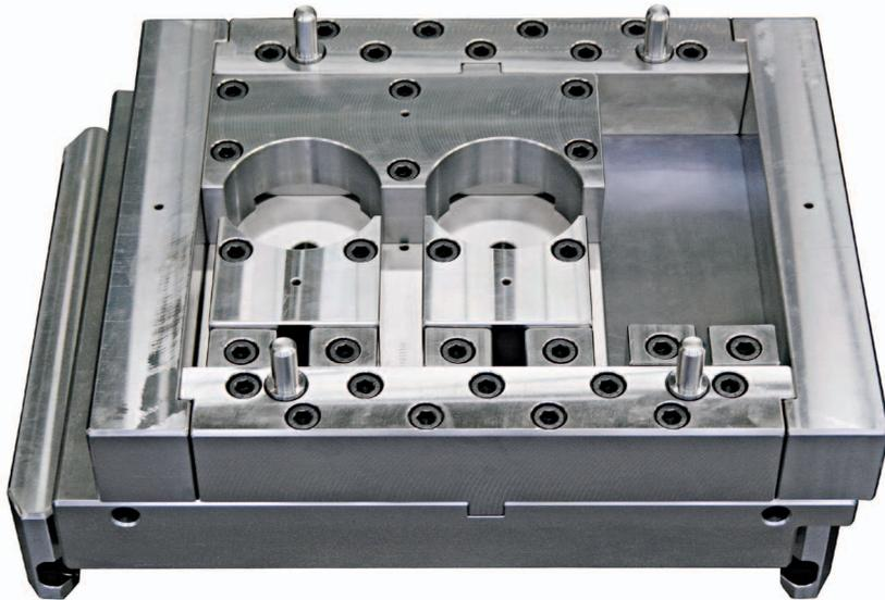
Rectangular forging die cassette lower section with 3 forging stations (from right to left: upsetting, preforming, finish-forging) and round forging die adaptation parts (view from front top)
