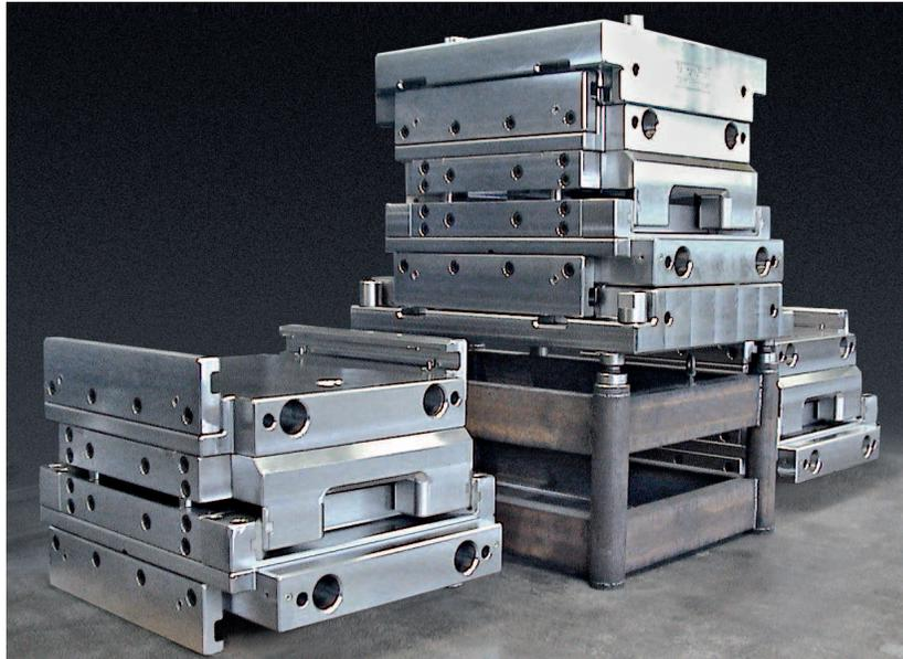
Base holder with installed rectangular forging die cassette on press bedplate dummy, base holder upper section in position "press ram at bottom", to the left and right ready-to-install complete rectangular forging die cassettes (view from front left)
