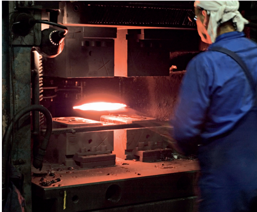
In forging use: die holder cassette quick-change system 08-25 with 3-station rectangular forging die cassette, here centrally equipped with 2 forging stations
