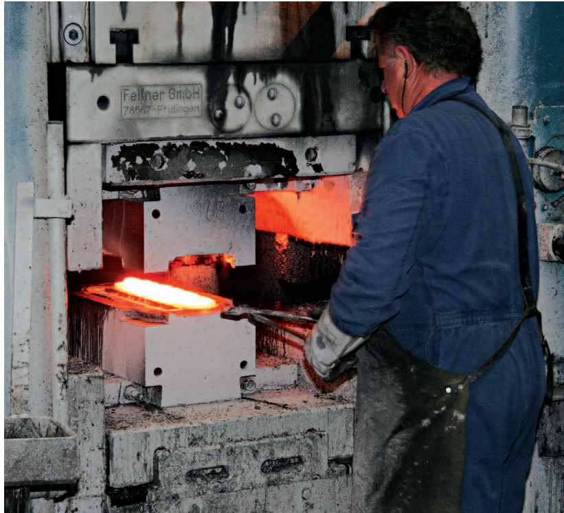
In forging use: dieholder cassette quick-change system 08-10 with 2-station dovetail forging die cassette, here equipped with one forging station
