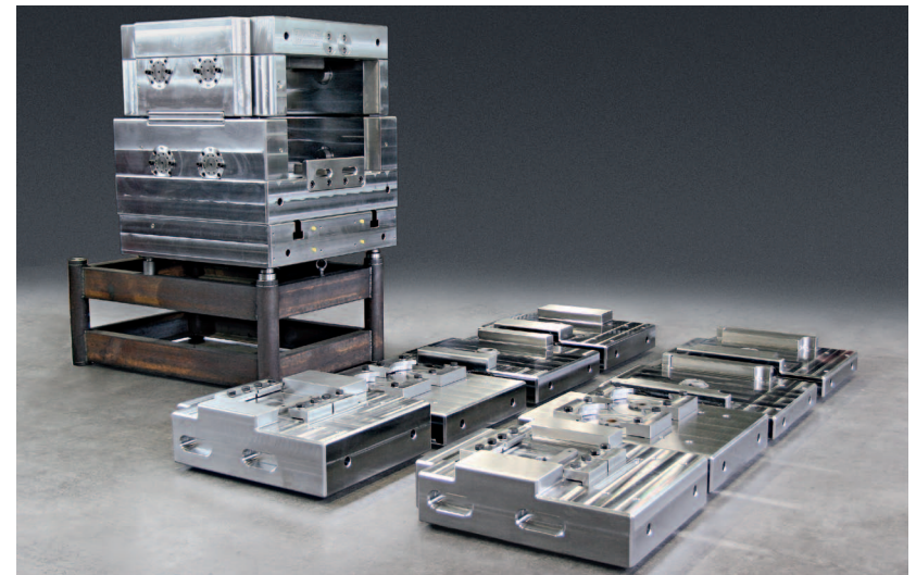
Base holder on intermediate plate and press bedplate dummy, base holder upper section in position "press ram at bottom", in front of which in each case one opened, ready-to-install, complete rectangular and round forging die cassette and two dovetail forging die cassettes (from left to right) (view from front left)
