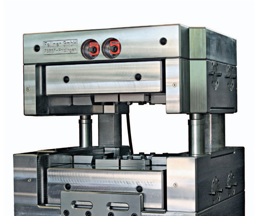
Base holder with flat/round pillar guide, mechanical-digital position indicators of the forging offset correction system and installed rectangular forging die cassette, base holder upper section in position "press ram ¾ at top" (view from front right)
