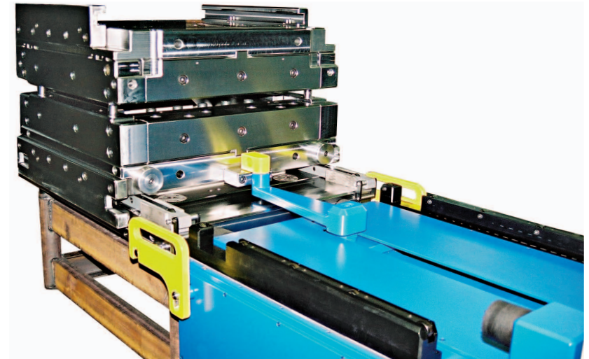
Cassette change carriage in cassette change position in front of the "press" (press bedplate dummy), ready-to-change rectangular forging die cassette on mobile Rollbloc roll blocks on the base holder lower section and coupled to the cassette coupler arm of the change carriage (view from front left top)
