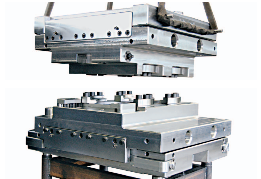
Base holder with installed, clamped round forging die cassette, base holder upper section in position "press ram at bottom" (view from front left)
