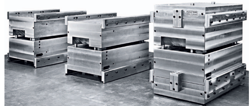
Base holder with installed, clamped rectangular forging die cassette, base holder upper section in position "press ram at bottom", to the left complete rectangular forging die cassettes ready for installation (view from front right)
