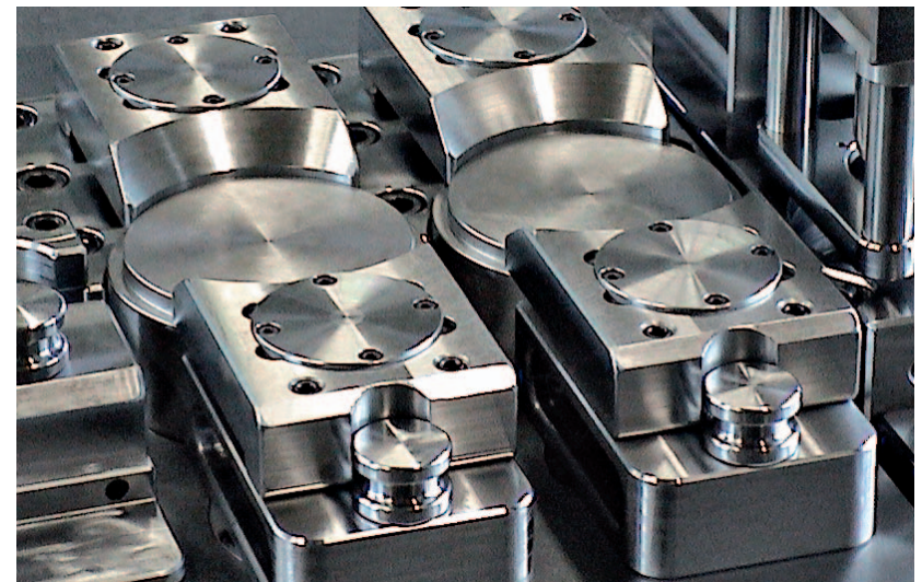
Double-hydraulic pull-down clamping elements in a round forging dieholder lower section of a Fellner forging die quick-change system for a 6.5 MN drop forging wedge press with clamped round forging die lower section dummies (view from front left top)
