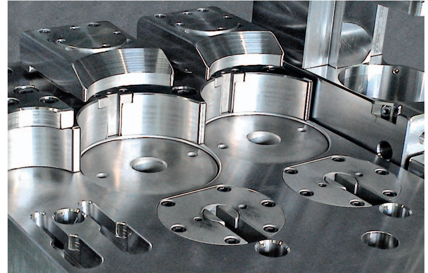
Double-hydraulic pull-down clamping elements, at front without pull-down rods and forging die clamping claws, in a round forging dieholder lower section of a Fellner forging die quick-change system for a 6.5 MN drop forging wedge press (view from front left top)
