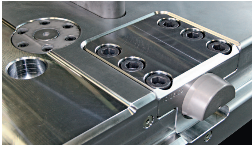
Hydromechanical wedge-type clamping element in a base holder lower section of a Fellner dieholder cassette quick-change system for a 16 MN drop forging eccentric press
