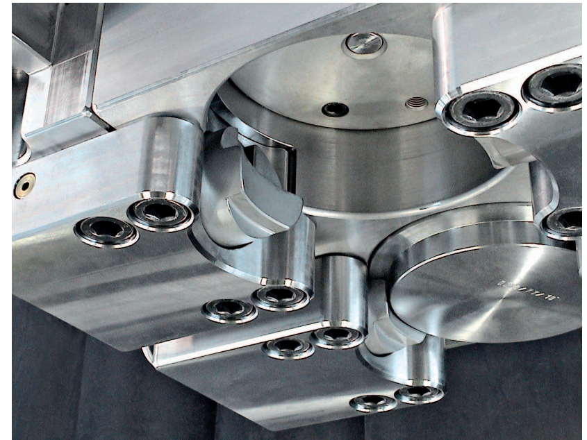
Hydromechanical wedge-type clamping elements in a round forging dieholder upper section of a Fellner forging die quick-change system for a 6.5 MN drop forging wedge press (view from rear right bottom)
